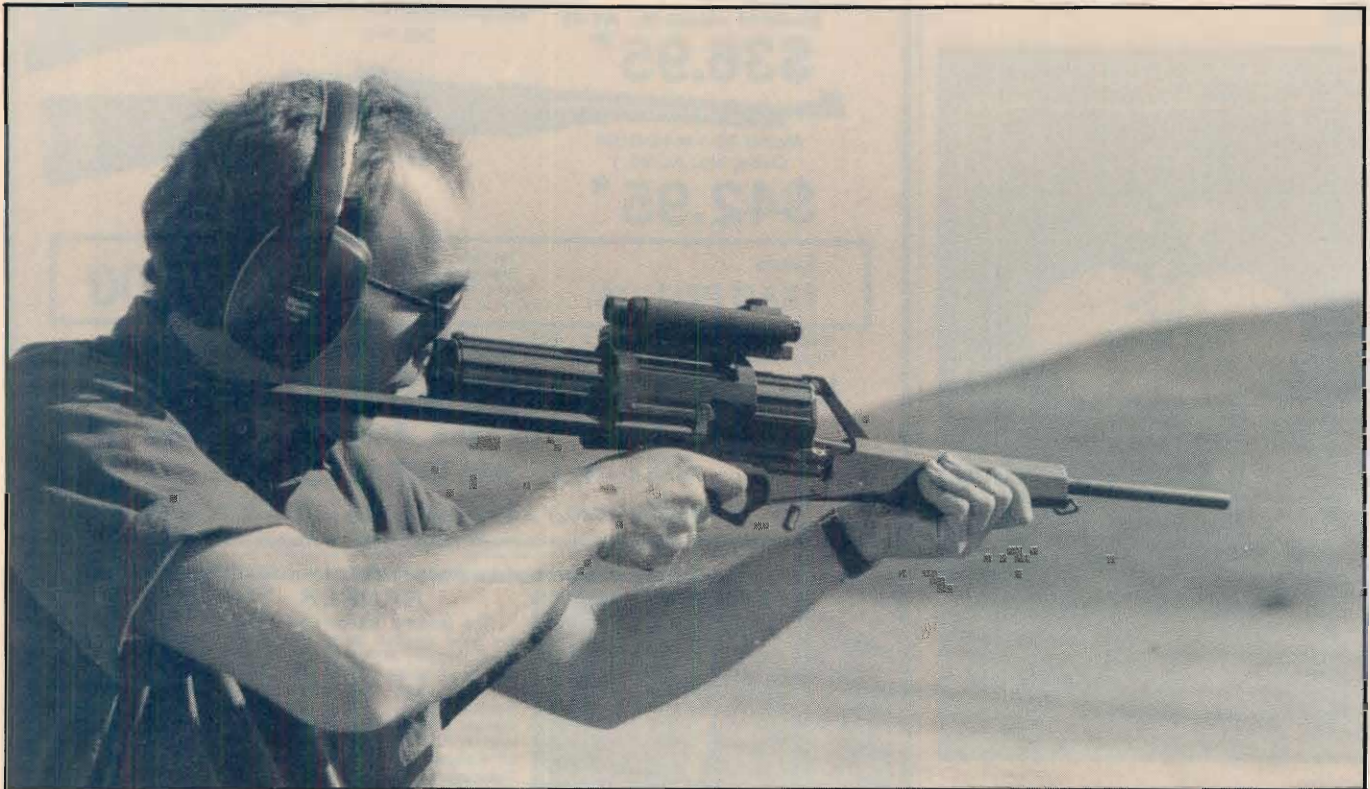
The M-900 Carbine being fired with stock extended. Cartridge cases are ejected downward from the ejection port in front of the trigger guard.
